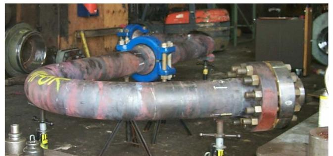
API 6A 5.1/8" 15M Flowline under hydro test at 22500 psi
