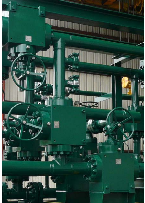
4" 15M CF Series Gate Valve (Full Port) – LTS Pigging System
