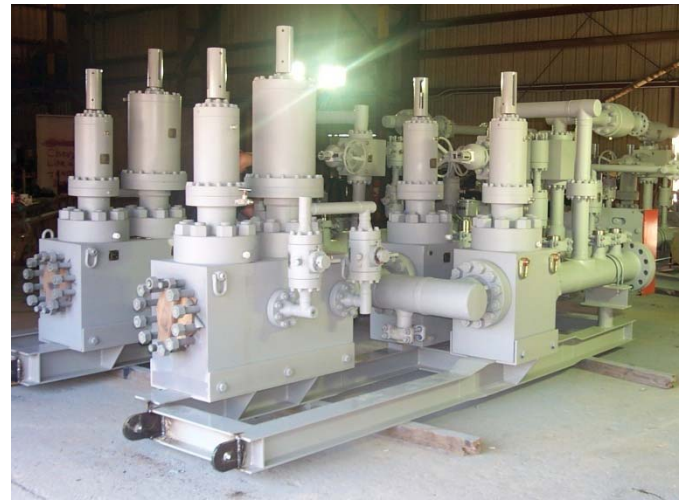
8" 15M CF Series Gate Valve (Exact Port) - LTS Pigging System
